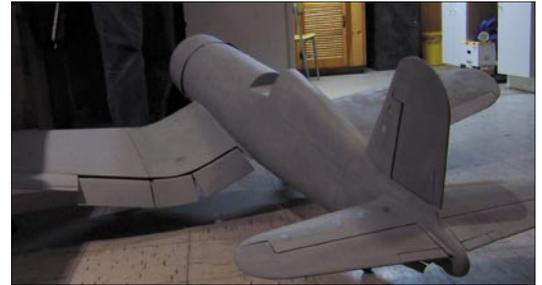
Paul Chaisson's giant corsair was built from a Byrons kit. Fiberglass fuse with sheeted foam wings.
